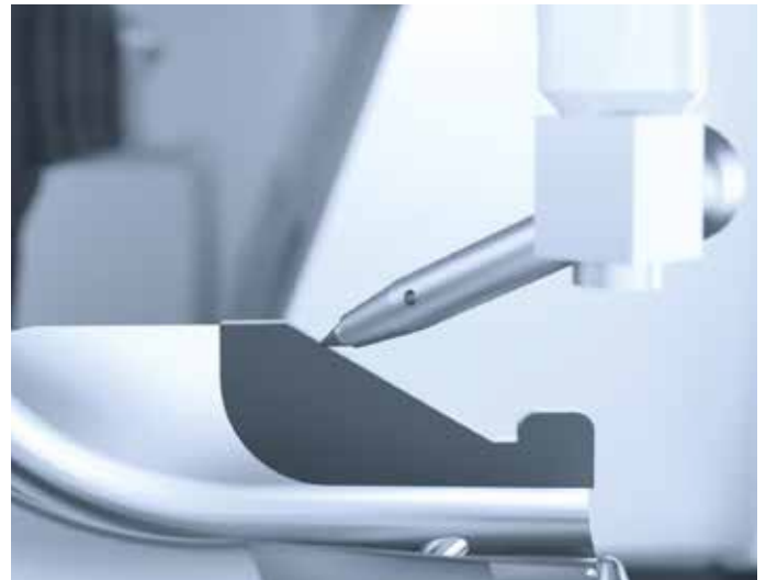
/// CONTOUR EDGE MEASUREMENT for precision machining
