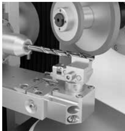
///// STEADY REST WITH AUTOMATIC STROKE Ensures an optimal grinding result for longer tools
