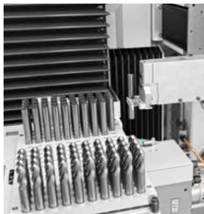
///// INTEGRATED PALLET LOADER With a capacity for up to 300 blanks or tools
