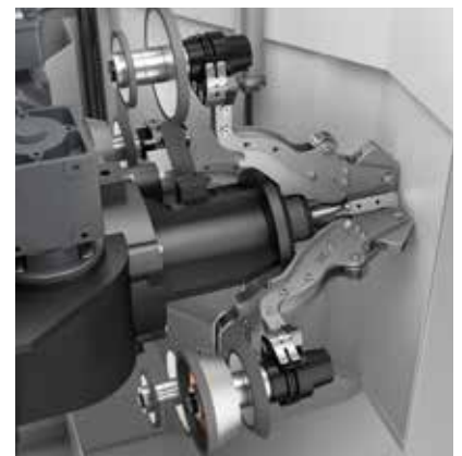
///// FOUR-STATION GRINDING-WHEEL CHANGER For efficient grinding wheel changes and the reduction of non-productive cycles
