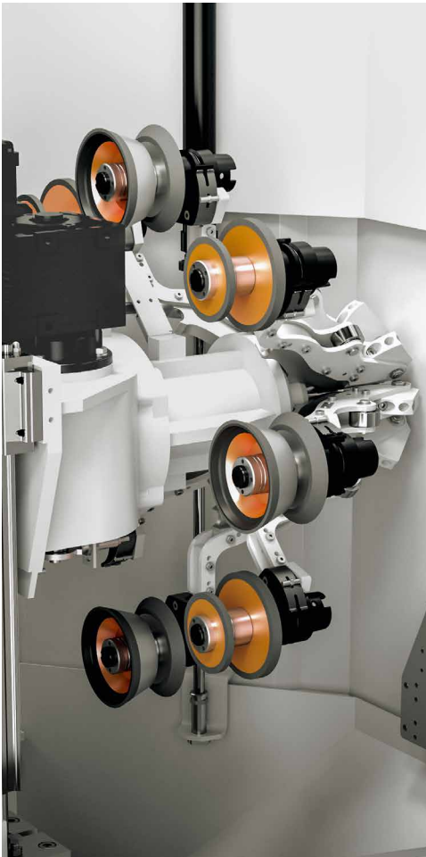
///// EIGHT-TOOL GRINDING-WHEEL CHANGER for efficient grinding wheel replacement and reduced non-productive time
