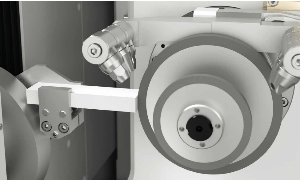
///// STICKING UNIT for opening the abrasive grinding wheel
