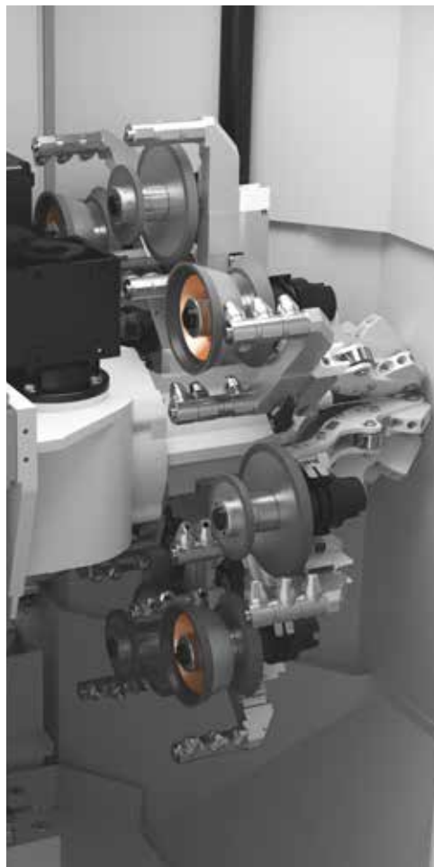
///// EIGHT-STATION GRINDING-WHEEL CHANGER including interchangeable coolant elements
