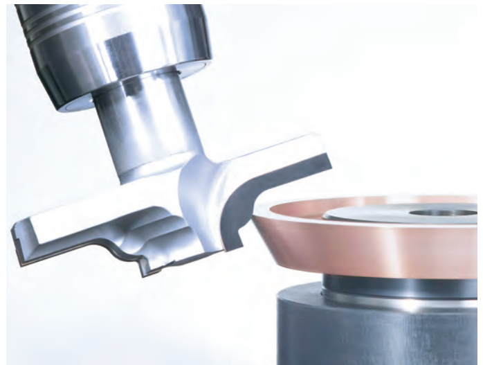
/// ERODING A PROFILED WORKPIECE
