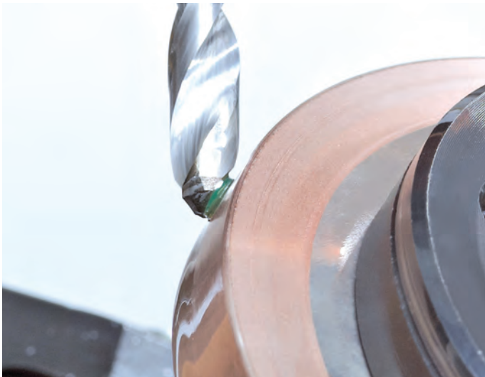
/// FLUTE EROSION of a PCD twist drill
