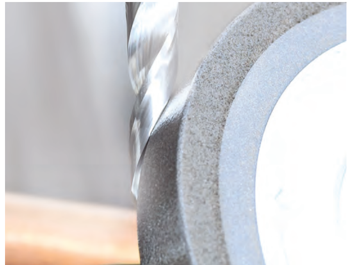
/// FLUTE GRINDING of a PCD twist drill
