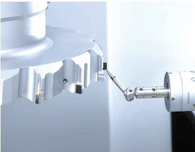
/// MEASURING THE CUTTING EDGES
