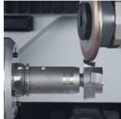
Eroding of a profile cutter with the peripheral rotary electrode.
