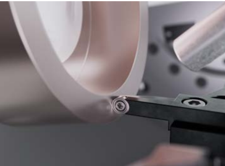
////// AUTOMATIC MEASURING AND DRESSING OF THE EROSION ELECTRODE
