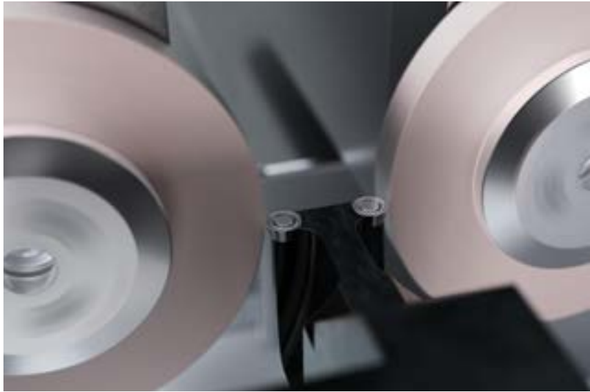
///// AUTOMATIC MEASURING AND DRESSING OF THE EROSION ELECTRODE
