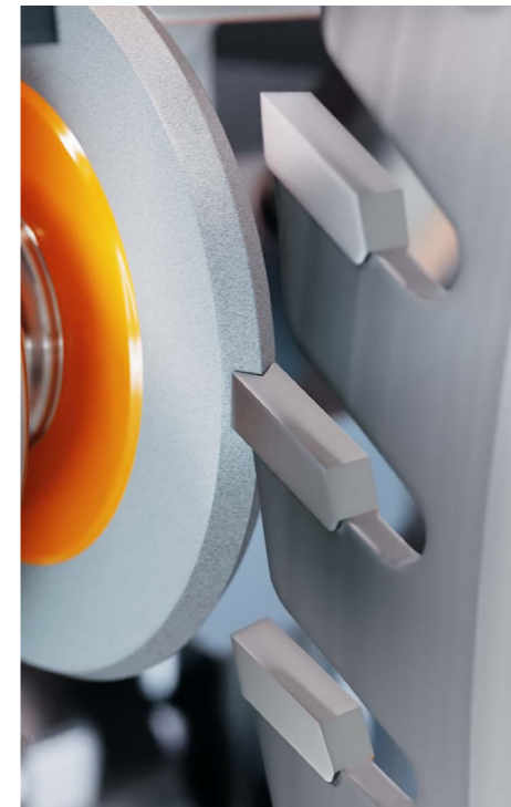
//////// MACHINING OF THE V-SHAPED GROOVE ON THE TOOTH TOP
