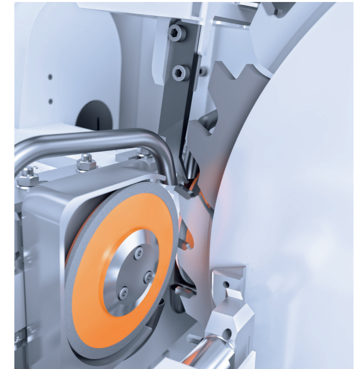
/// MACHINING A CHIPPER SEGMENT from the saw mill industry
