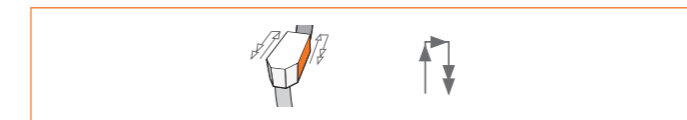
/// GRINDING PROGRAM Grind forwards, lift off, followed by a rapid traverse movement
