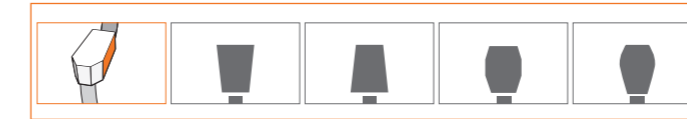
/// SIDE ANGLE // MACHINABLE TOOTH PROFILE EXAMPLES Convex tooth flanks, positive/negative radial angles (e.g. prescoring circular saws)
