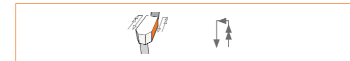
/// GRINDING PROGRAM A rapid forwards movement, feed, followed by a grinding pass back again
