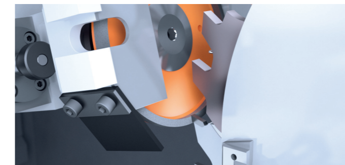
/// TOOTH TOP MACHINING on chipper segment from the saw mill industry
