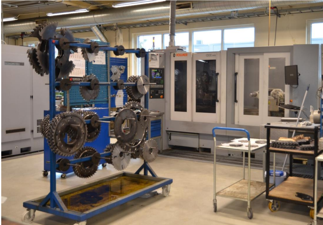
Caption: Kvarnstrand uses around 50 Vollmer machines in service, including a CHC 840, CHX 840 and CHD 270 for the automated machining of carbide-tipped circular saws used in the processing of wood, aluminium and plastic.
