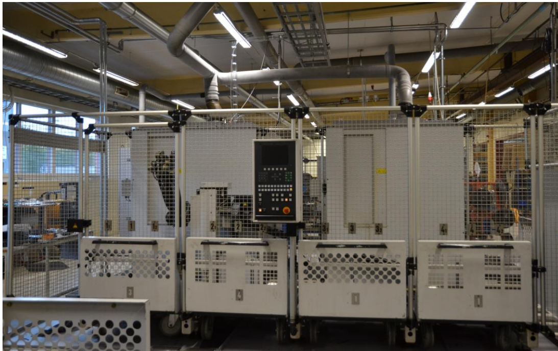
Caption: Thanks to the Vollmer ND 340 handling system with its four loading carriages, Kvarnstrands can automatically load grinding machines with up to 350 circular saw blades.
