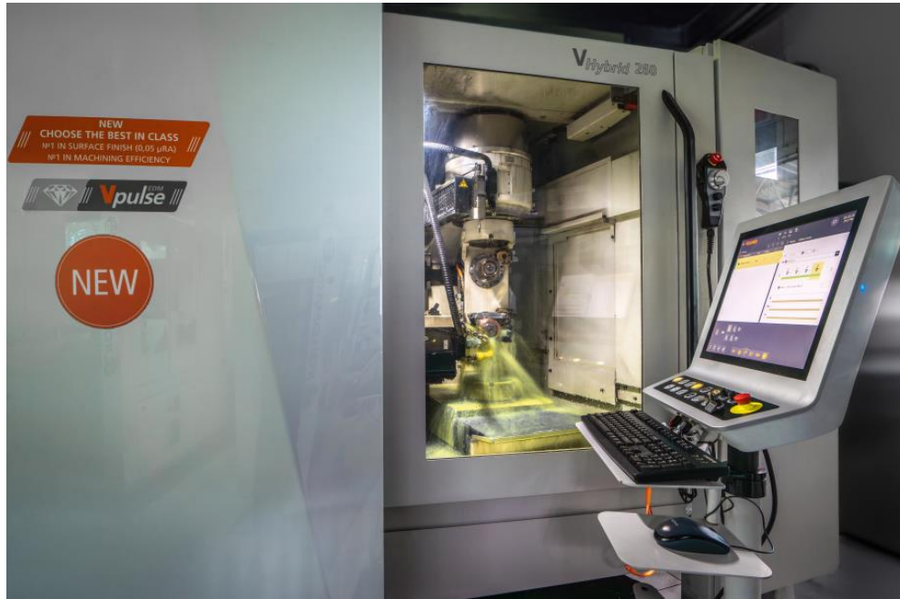
Caption: N.S.T. Machinery can use the VHybrid 260 VOLLMER grinding and erosion machine to grind or erode up to 100 per cent of both carbide and PCD tools.
