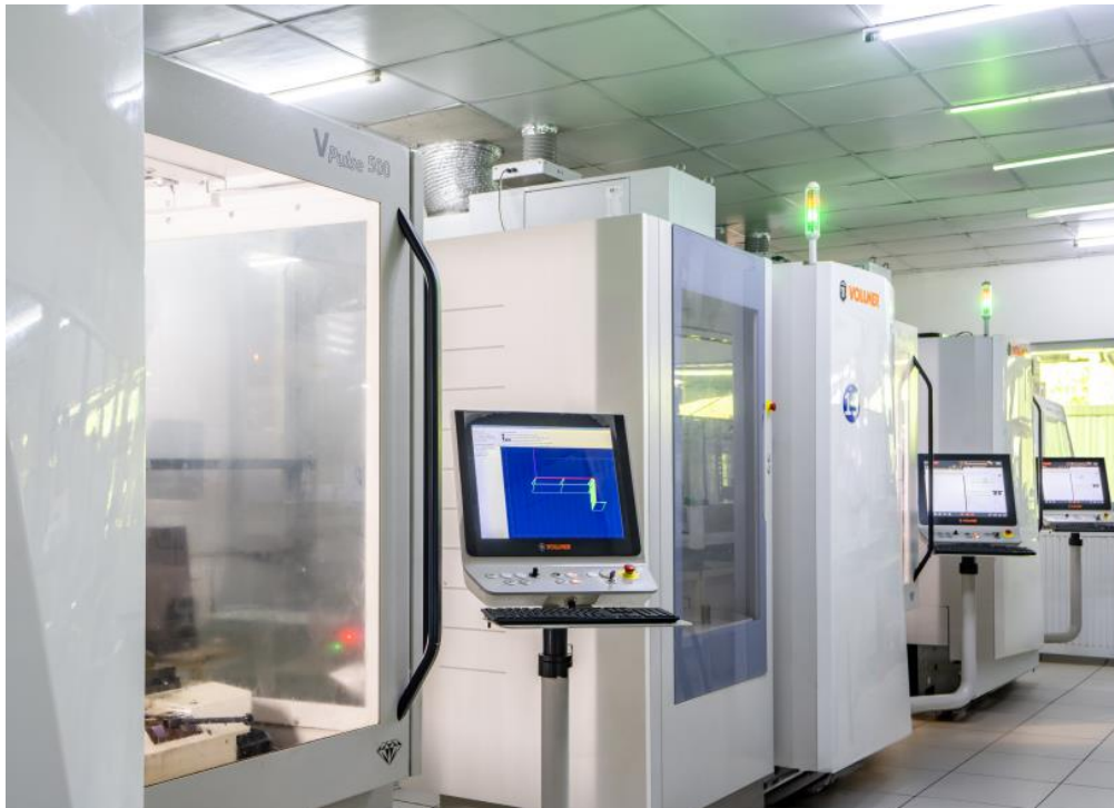
Caption: Five VOLLMER wire erosion machines are in operation at the Thai tool manufacturer N.S.T. Machinery, and form the basis of the enormous growth in PCD-tipped tools.
