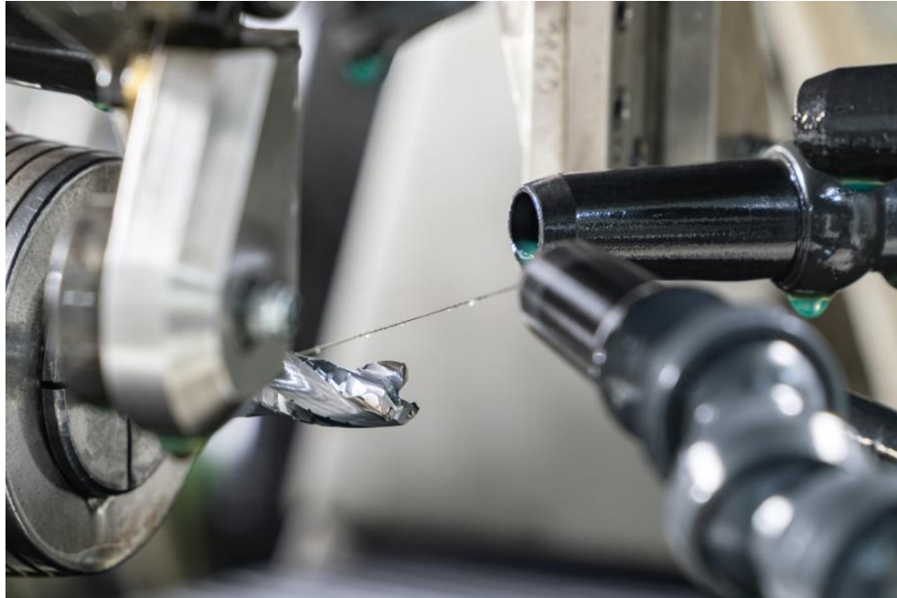
Caption: Due to the wire, N.S.T. Machinery can use the VOLLMER VPulse 500 erosion machine for precise machining even of complex geometries and small inner radii – these structures are typical of multi-stage tools and bell-shaped tools.
