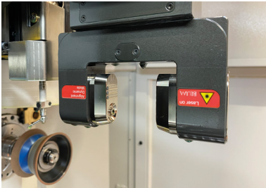
// CLOSED LOOP AT CYLINDRICAL EROSION to achieve tight diameter tolerances
